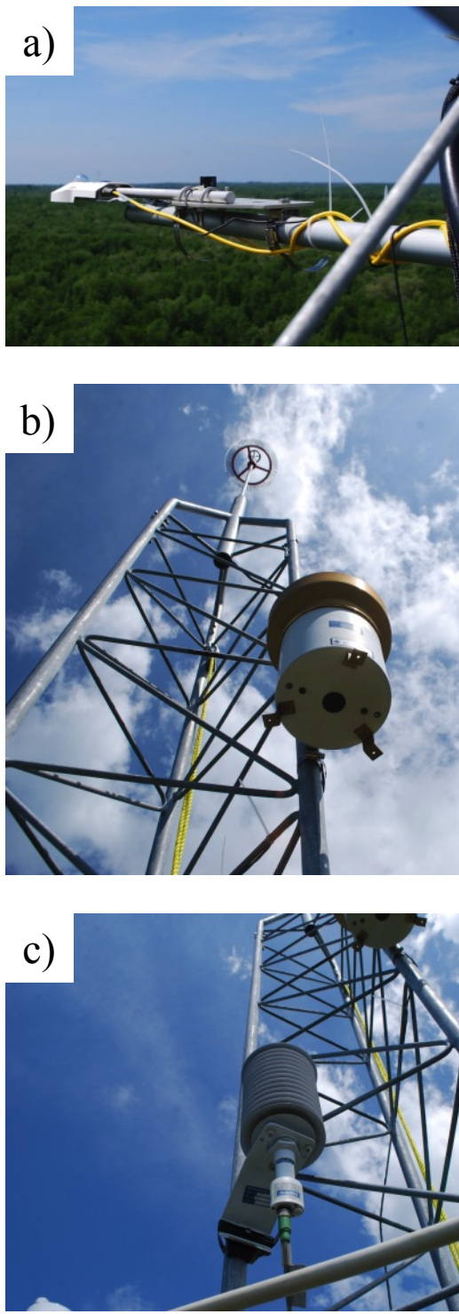
Figure 18. Meteorological sensors including: a) 4 way radiation sensor for long and shortwave incoming and outgoing, and photosynthetic active radiation sensor; b) rain gauge; c) relative humidity and air temperature sensor.
